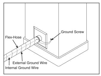
Figure 16. Flex-hose grounded to machine.
